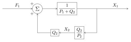
Altogether the feedback branch, along the bottom, multiplies  $X_1$  by  $Q_2^2/P_2$ . Notice that the feedback is entirely determined by the parameters of the secondary oscillator.
