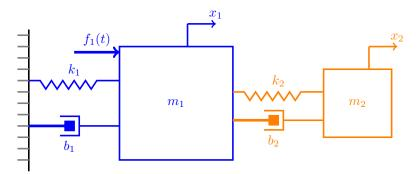
We will regard first mass as the building, or the table – it's being shaken by some force, and we wish to control the ampitude of its resulting oscillation – so the system response of interest is  $x_1$ . The second mass is presumably smaller, and the behavior of  $x_2$  is of only secondary interest.
