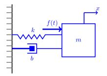
We get different equations if the force is applied to the spring or the damper instead of the mass. We can get more complicated systems by coupling together two or more spring-mass systems.
