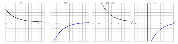
When the time invariant system is also linear we call it a linear time invariant system. We abbreviate this by calling it an LTI system.
