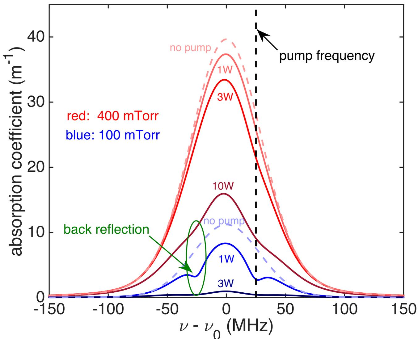
Fig. S1. IR absorption spectrum at 100 mTorr and 400 mTorr with various input pump powers.  $\nu_0 = 31.0427$  THz is the frequency of the L-U transition, while the  $\text{CO}_2$  pump laser is incident at a frequency 25 MHz  $>$   $\nu_0$ .
