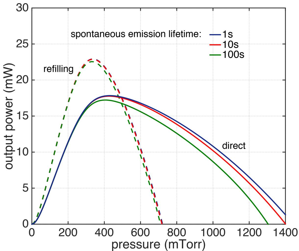
Fig. S7. Numerical output power of both direct (solid lines) and refilling (dashed lines) lasing versus pressure with the input pump power equal to 10W, and with three different spontaneous emission lifetimes  $t_{sp}$ : 1sec, 10sec, and 100sec.  $t_{sp}$  has little effect on the peak output power far above threshold for both lasing transitions.
