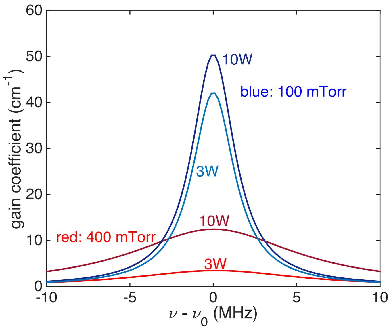
Fig. S6. THz gain spectrum at 100 mTorr and 400 mTorr with the input pump power equal to 3W and 10W. The width of spectrum is proportional to the gas pressure due to pressure broadening.
