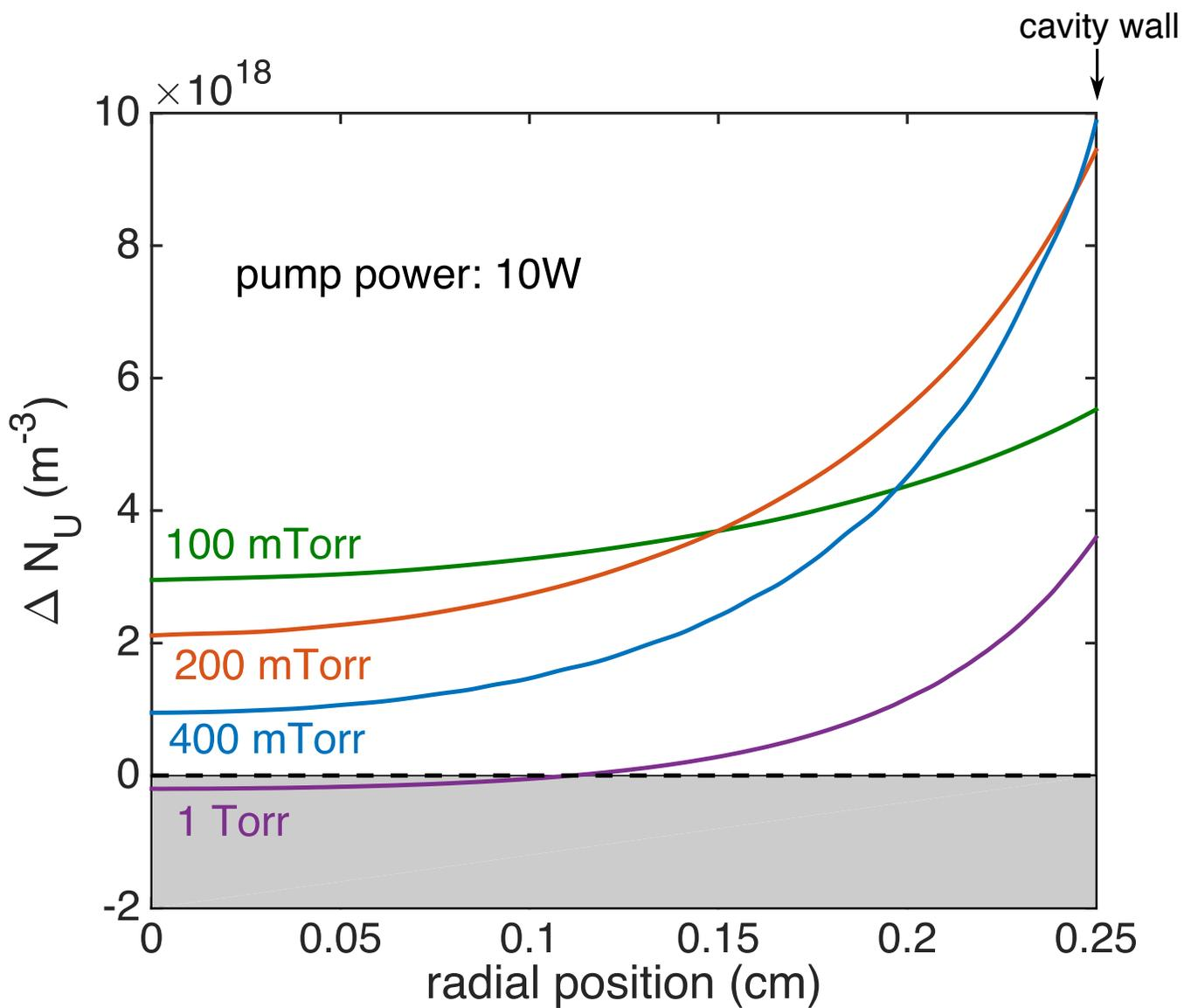
Fig. S3. Radial distribution of population inversion for direct transition at 100 mTorr, 200 mTorr, 400 mTorr, and 1 Torr, with 10W input pump power.
