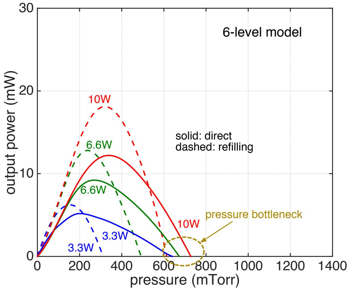
**Fig. S2.** THz output power as a function of gas pressure, for various input pump powers (3.3W, 6.6W, and 10W), and for both the direct (solid lines) and refilling (dashed lines) transitions by a 6-level model. It is clearly observed that no gain is obtained above 700 mTorr by the 6-level model, known as high-pressure unphysical bottlenecking.
