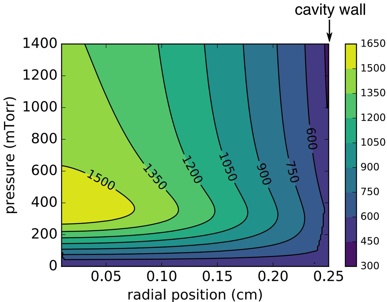
**Fig. S4.** The effective temperature  $T_v$  (in Kelvin) of type-A vibrational thermal pools as a function of radial position and molecular pressure, for an input pump power of 10W. The cavity is 5mm  $\times$  14.3cm as in experiments.
