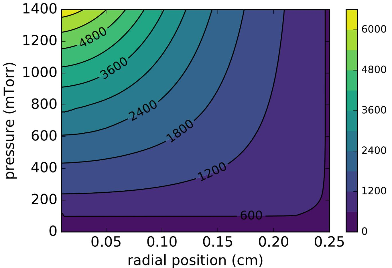
Fig. S5. The effective temperature  $T_v$  (in Kelvin) of type-A vibrational thermal pools as a function of radial position and molecular pressure, for an input pump power of 10W. The cavity length is optimized to match the IR absorption:  $L_o = 1/2\alpha_p$ , and the cavity diameter is 5mm.
