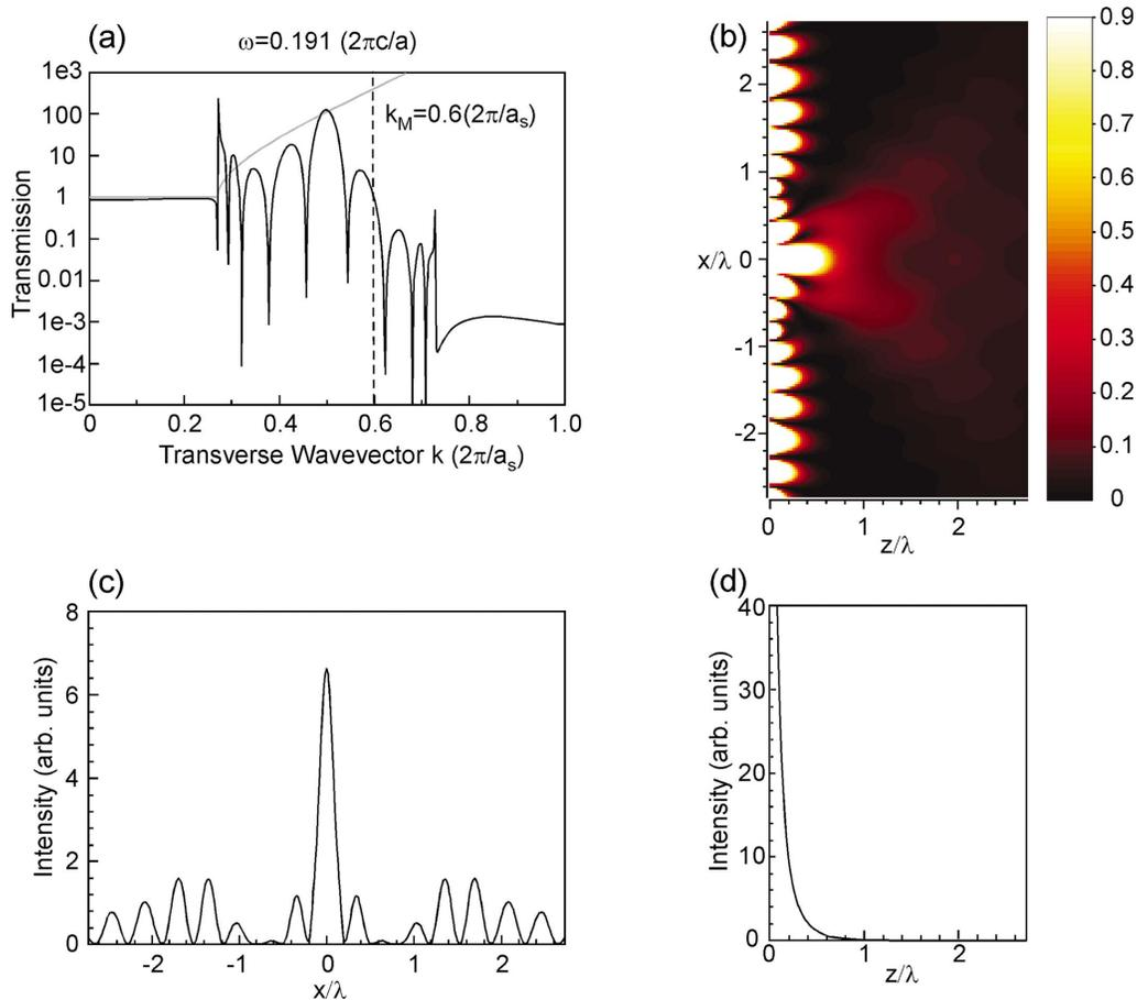
FIG. 7. (Color) Numerical results similar to those shown in Fig. 5 for  $\omega=0.191 (2\pi c/a)$ . (c) is a plot in the plane of  $z=a_s=0.27\lambda$  (not through an intensity maximum).
