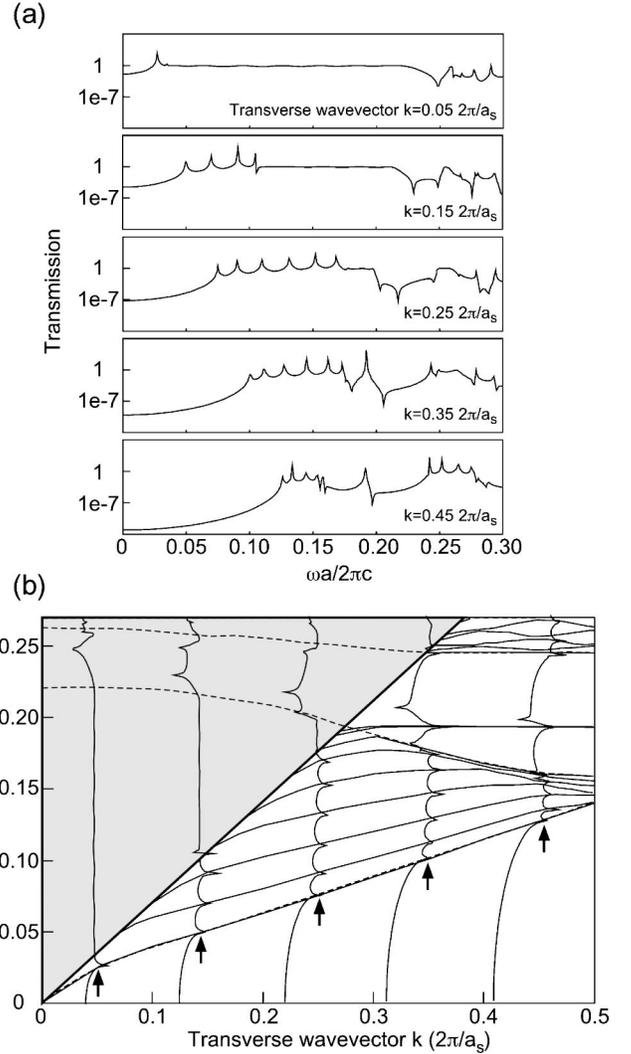
FIG. 4. Frequency spectrum of transmission and links to bound slab photon modes. (a) Zeroth-order transmission ( $|t_{00}|^2$ ) through the photonic-crystal slab in Fig. 3 for various transverse wave vectors, plotted on a logarithmic scale vs frequency. (b) The transmission curves in (a) are plotted on the bound photon band structure of the photonic-crystal slab [Fig. 3(a)]. The arrows indicate the transverse wave vector for each transmission curve. The shaded region is the light cone.
