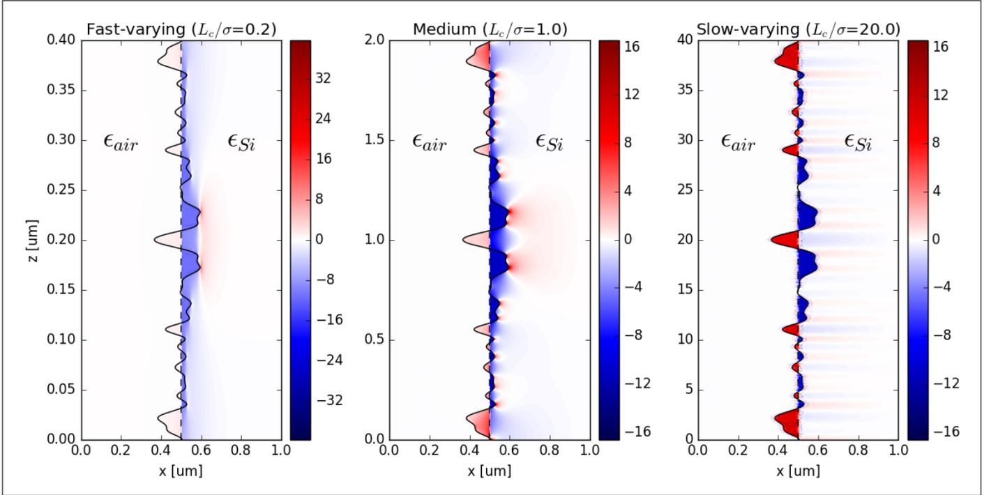
**Fig. S1.** Computed changes in the perturbed polarization density  $\Delta P(\vec{r}) \cdot \hat{z}$  along a rough waveguide sidewall with short ( $L_c/\sigma = 0.2$ ), medium ( $L_c/\sigma = 1.0$ ), and long ( $L_c/\sigma = 20$ ) correlation lengths with respect to the RMS roughness  $\sigma$ . Solid black line shows the perturbed sidewall, and dashed black line shows the straight, unperturbed sidewall.
