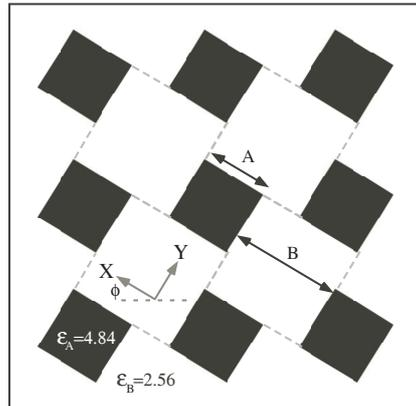
**Figure 1.1.** Unit cell of the Fibonacci superspace dielectric. The physical dielectric is obtained by taking a slice at an angle  $\tan \phi = \tau$ . Black/white are the dielectric constants of the structure factor material and air, chosen to be  $\epsilon = 4.84$  and  $\epsilon = 2.56$ , respectively.
