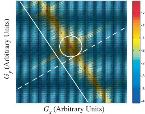
**Figure 1.7.** Fourier-space spectrum  $|\mathbf{H}_G|^2$  of a physical mode, on a log scale. In contrast to Fig. 1.6., the primary support of this mode occurs in the center of the computational cell.
