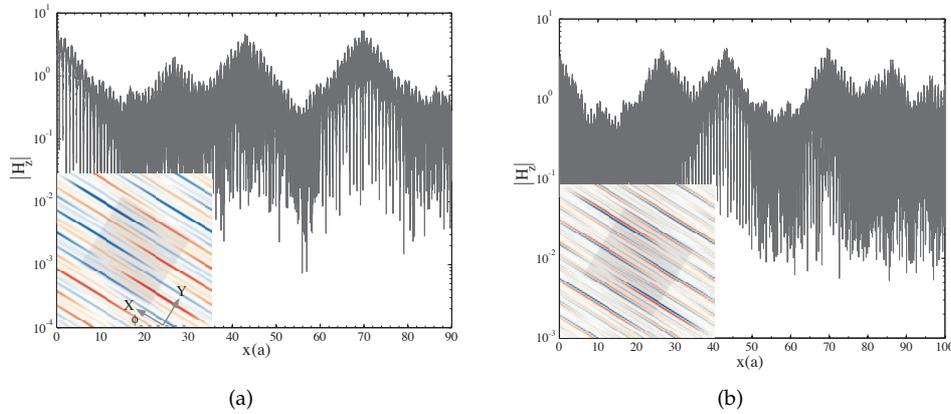
**Figure 1.12.** Semi-log plots of the magnetic field magnitude  $H_z$  for the lowest (a) and highest (b) defect state for the configuration shown in Fig. 1.10.. *Insets:* Two-dimensional superspace visualizations of the defect states. Note the additional node in the lower figure (corresponding to an unphysical oscillation).
