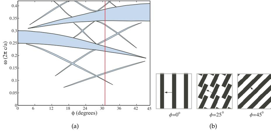
**Figure 1.13.** Projected bandstructure vs. cut angle  $\phi$ , showing different one-dimensional quasicrystal realizations. The vertical red line indicates the spectrum when the slope is the golden ratio  $\tau$  (the spectra of  $\phi$  and  $\pi - \phi$  are equivalent)
