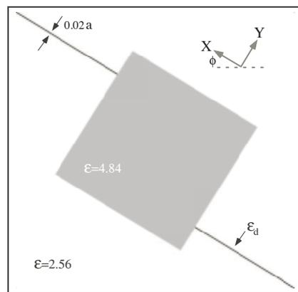
**Figure 1.10.** Dielectric for the Fibonacci chain with  $\epsilon = 2.56$  (light blue), and a defect—an additional  $\epsilon_d = 8.0$  layer, shown in gray.
