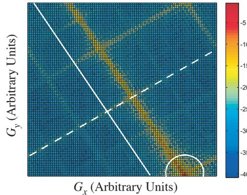
**Figure 1.6.** Fourier-space spectrum  $|\mathbf{H}_G|^2$  of a spurious mode, on a log scale: dashed white line denotes the “physical” X direction in which fluctuations carry an energy penalty, and the solid white line denotes the “un-physical” Y direction. Circle denotes the peak in the mode’s Fourier-space support, which occurs at the boundary of the computational cell.
