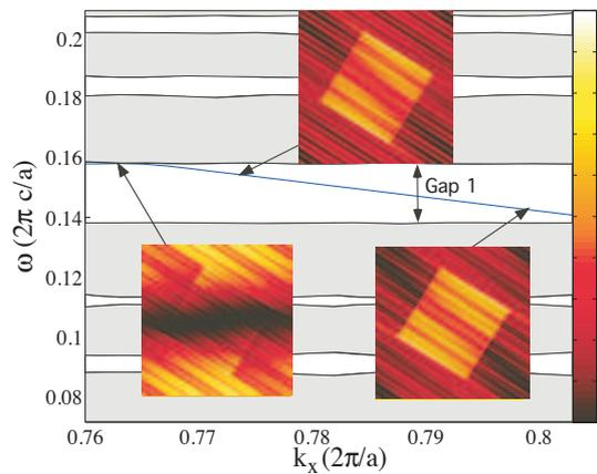
**Figure 1.4.** Enlarged view of the Fibonacci spectrum showing a gap with a spurious band crossing it. Insets show the magnetic field  $|H_z|$  for the spurious band at various  $k_x$ —the localization of this mode around the X-parallel edges of the dielectric indicate that this is a discretization artifact.
