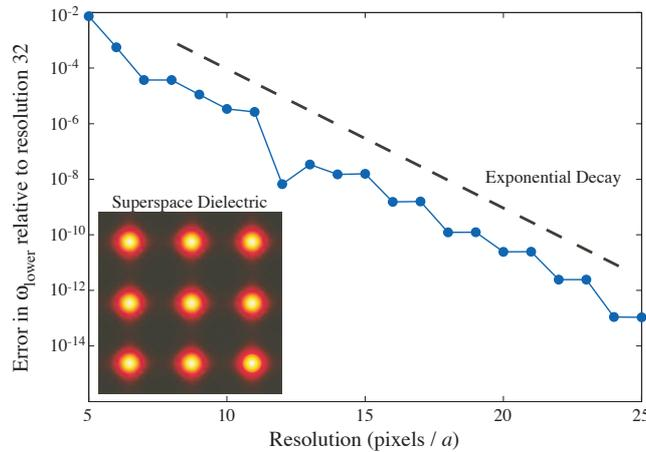
**Figure 1.15.** Demonstration of exponential convergence with resolution of a smooth superspace structure. A plot of the error in  $\omega_{\text{lower}}$  from Fig. 1.14. (relative to resolution 32) shows exponential convergence. The superspace dielectric structure, given by Eq. (1.4), is shown in the inset.
