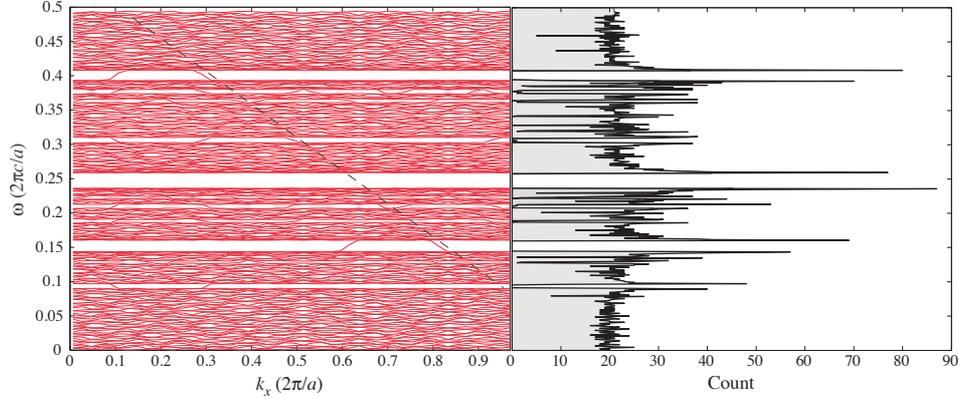
**Figure 1.5.** Identification and removal of spurious modes in one dimension. Left: spectrum of the Fibonacci quasicrystal, as in Fig. 1.3.. We have superposed a black dashed line to indicate that the spurious modes appear to largely follow a linear dispersion relation. Right: density-of-states computed by removing all modes that satisfy  $\lambda(\mathbf{H}) \geq 0.9$ , where  $\lambda$  is defined in Eq. (1.3). All spurious modes in the large bandgaps have vanished.
