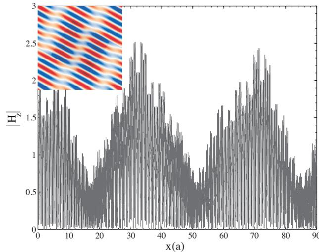
**Figure 1.8.** Plot of the magnetic field amplitude  $|H_z|$  for a band-edge state taken along a slice of the two-dimensional superspace (in the  $\phi$  direction). *Inset:* Two-dimensional superspace field profile (red/white/blue indicates positive/zero/negative amplitude).
