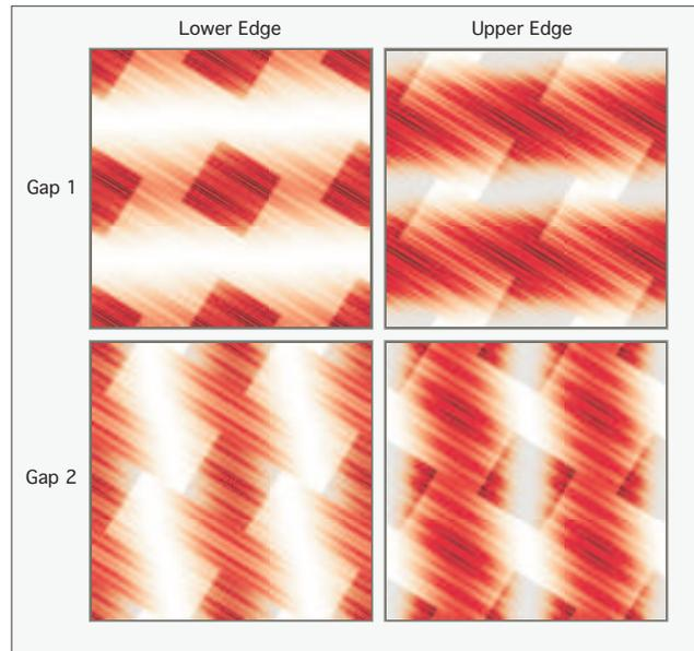
**Figure 1.9.** Electric field energy distribution of the band edge states of gaps 1 and 2 in Fig. 1.3.. Although they have a complex small-scale structure, the large-scale variation is easily understood in terms of the structure of the superspace.
