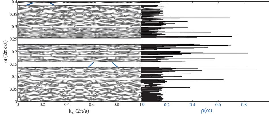
**Figure 1.3.** *Left:* Frequency spectrum  $\omega$  of the Fibonacci quasicrystal vs. “wave-vector”  $k_x$ . The blue lines indicate spurious states which arise due to finite resolution effects (see text). *Right:* Corresponding density of states  $\rho(\omega)$  computed using a transfer-matrix technique with a supercell of  $10^4$  layers.
