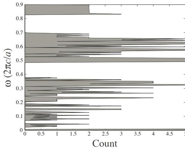
**Figure 1.18.** Mode density plot for the superspace octagonal structure, with the same structural parameters as Fig. 1.17., for a resolution of 10 pixels per  $a$ . At this resolution, the bandgaps are not fully resolved to high accuracy.
