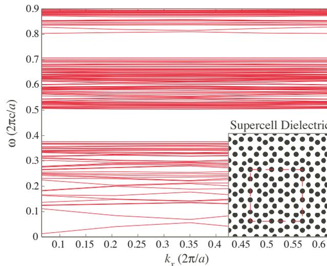
**Figure 1.17.** Bandstructure for a  $3/2$  supercell approximate to the octagonal PQC of high dielectric rods. The real-space structure is shown in the inset, with a unit cell marked by the dashed red box.
