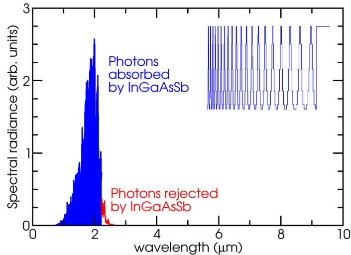
Fig. 5. (Inset) Chirped rugate filter index as a function of position (using 6 materials) and (Main image) its emittance as a function of wavelength. Emitted photons with wavelengths  $\lambda < 2.23 \mu\text{m}$  (depicted in blue) are capable of being absorbed by the InGaAsSb TPV device.
