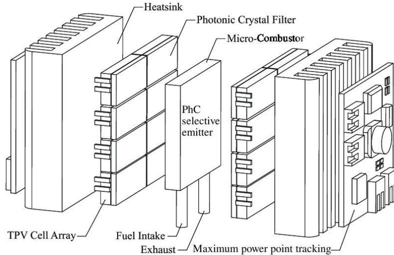
Fig. 2. Design of the  $\mu$ TPV generator. Hydrocarbon fuel flows from a storage tank to the interior of the selective emitter and back out. The heated selective emitter then radiatively couples to the nearby TPV module to generate electricity (adapted from Ref. 31).
