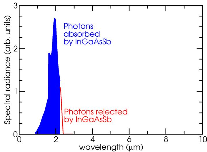
Fig. 8. Spectral emittance for combined tungsten 2D PhC and rugate filter. Emitted photons with wavelengths  $\lambda < 2.23 \mu\text{m}$  (depicted in blue) are capable of being absorbed by the InGaAsSb TPV device.
