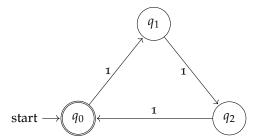
For arbitrary *n*, we want a cycle like the above, but consisting of *n* states, representing the length being 0, 1, ..., n - 1 modulo *n*. *M* =  $(Q, \Sigma, \delta, q_0, F)$  recognizes  $A_n$ , where
