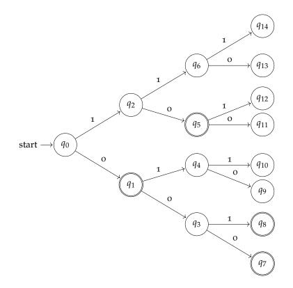
In additiona, there is an dead state from which states  $q_7$ , ...,  $q_{14}$  lead to on any input, since we don't want to accept any strings of length longer than 3. We haven't drawn the dead state or its associated transitions to simplify the diagram.
