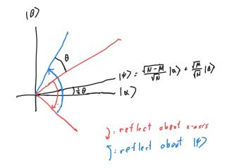
If the two reflections are about lines that intersect at an angle of  $\phi$  radians, then their product is a rotation around the intersection by an angle of  $2\phi$  radians. Thus, each Grover iteration rotates the state by approximately  $2\frac{\theta}{2} = \theta \approx 2\frac{\sqrt{M}}{\sqrt{N}}$  radians. We would like the state to be rotated to the axis  $|\beta\rangle$ , which is at an angle of approximately  $\pi/2$ from the original state  $|\phi\rangle$ . This will take roughly
