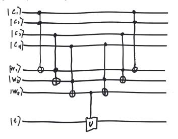
Here, we use k - 1 extra work qubits which start in the state  $|0\rangle$ . If all the control bits are  $|1\rangle$ , then the first k - 1 Toffoli gates set all the work qubits to  $|1\rangle$ , and a controlled-U gate applied to the last work bit applies a U to the target qubit. Otherwise, the last work qubit remains in the state  $|0\rangle$ , and an identity is applied to the target qubit. The
