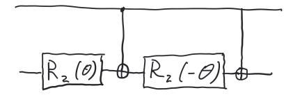
If the first qubit is a  $|0\rangle$ , then we have  $R_z(-\theta)R_z(\theta)$  applied to the second qubit, and these two operations cancel each other out. If the first qubit is  $|1\rangle$ , we have  $R_z(\theta)$ applied to the second qubit, followed by  $\sigma_x R_z(-\theta)\sigma_x$ . This is  $R_z(\theta)$ , which when multiplied by the first  $R_z(\theta)$  gives  $R_z(2\theta)$ . We thus have a circuit for a C- $R_z(2\theta)$ .
