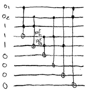
This took 6 Toffoli gates. To remove the work bits, we need four copies and then run the circuit in reverse. This piece takes 16 Toffoli gates. Call this  $C_2$ .
