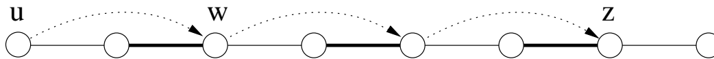
Figure 2.2: An augmenting path. Thick edges are in the matching. The path is found by starting from the exposed vertex u and following the dotted lines until a vertex (here z ) adjacent to an exposed vertex is found.
