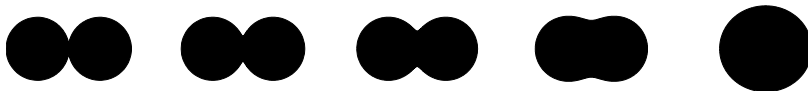
Figure 5. Evolution of the solution of Hopper [32] for the coalescence of two equal blobs of fluid under the effects of surface tension.
