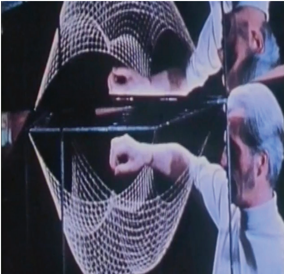
FIGURE 2. Architect and structural engineer Frei Otto pioneered the concept of “form finding”. Here he is experimenting with stable structures. To the right his famous olympic stadium based on his experiments with soap films.
