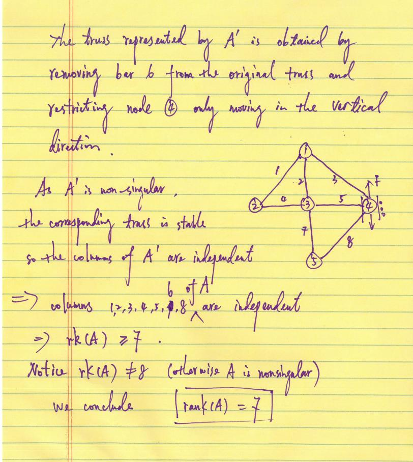
(3) As rank (A) = 7, its null space is of alimension 8-rank (A) = 1, consisting of the rigid motion described in So truss D in (1) does not have any
