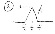
if  $J(x) = \alpha_i f_i(x) + \dots + \alpha_n f_{n-1}(x) = 0$   $J(\frac{i}{n}) = \alpha_i = 0$ . Therefore the  $f_i$ 's one independent.  $K_{ii} = 2n - \frac{4}{3n}$  for  $i = 4 - \dots n - 1$   $K_{i,i+1} = -n + 1 - \frac{1}{6n}$  for  $i = 1 - \dots n - 2$   $K_{i+1,i} = -n + 1 - \frac{1}{6n}$  for  $i = 2 - \dots n - 2$ all the other coefficients one O.
