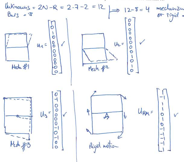
(b) (5 points) In Truss #1, add (draw) the minimum number of bars necessary to block all the mechanisms.
