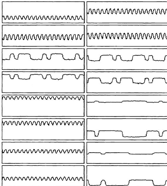
**Figure 3.** Optical oscilloscope traces from high-speed modulators for 1Gbit/s data and 1GHz square waves.
