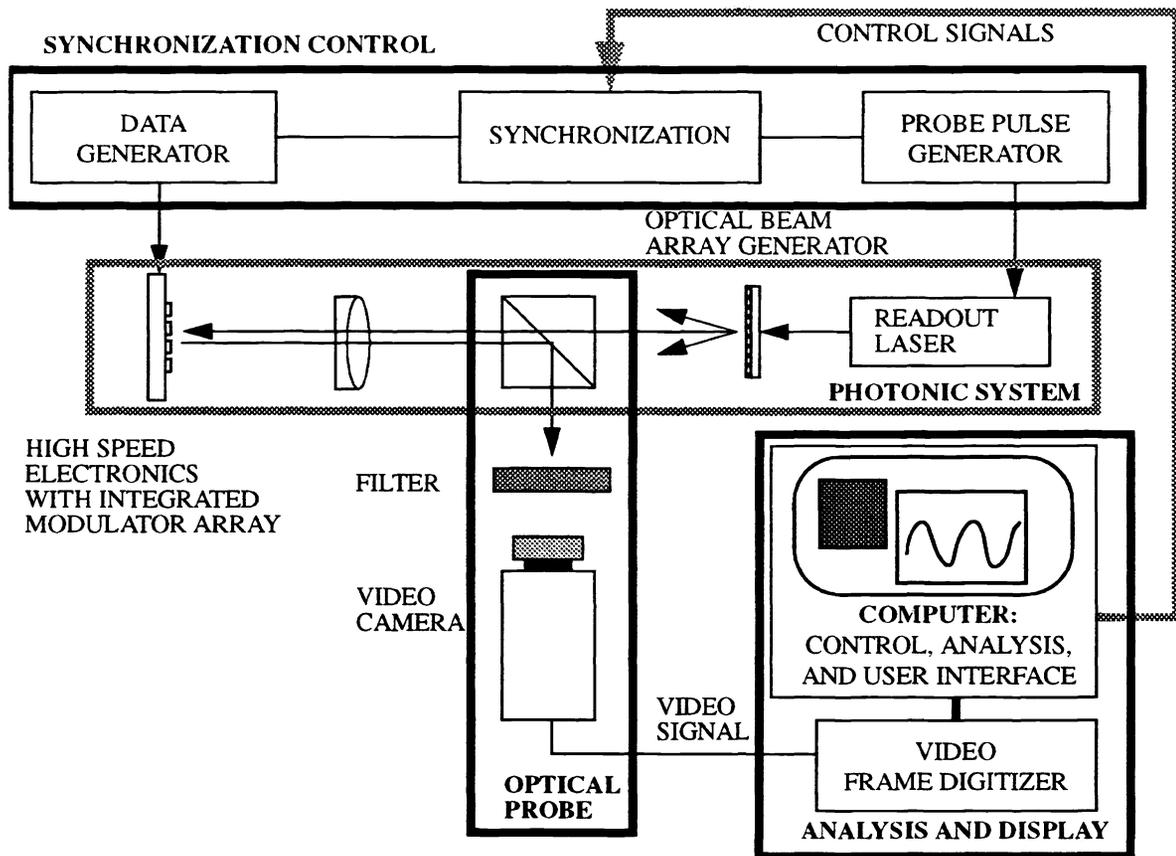
**Figure 1.** Schematic of test photonic system and optical oscilloscope modules.
