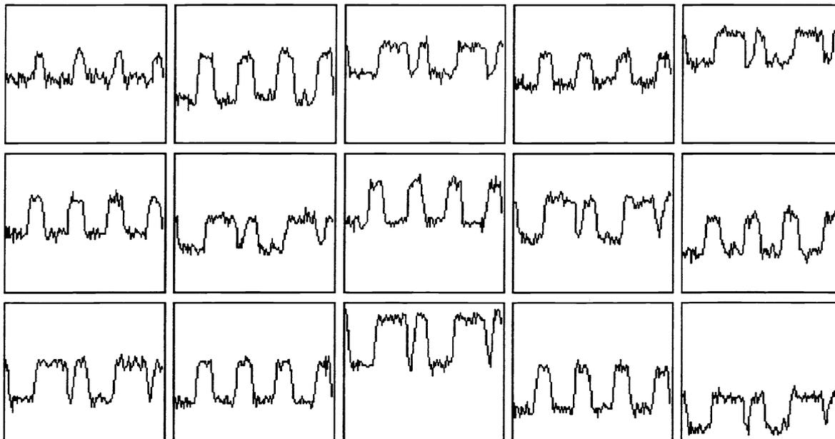
**Figure 4.** Fifteen traces obtained simultaneously from free-space photonic switch operating at a channel rate of 200 Mbits/sec. One of two separate input data channels is routed to each output modulator.
