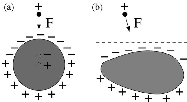
Fig. 1. (a) Electrostatics of a point charge interacting with a neutral metallic sphere. By using image charges (dotted circles), it is easy to see that the force  $\mathbf{F}$  on the point charge is attractive. (b) We ask whether the force is attractive for any shape of metallic object. More precisely, if the point charge and the object are on opposite sides of the  $z = 0$  plane (dotted line), with the charge in  $\{z > 0\}$  and the object in  $\{z < 0\}$ , is  $F_z$  always negative?
