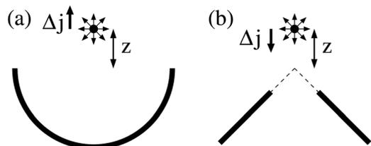
Fig. 8. (a) If current is injected into a homogeneous resistive sheet with conductivity  $\sigma$ , current flows from the injection point in a radially symmetric way. Reducing the resistivity to 0 in a thin semi-circular region causes an increase,  $\Delta j$ , in the current flowing away from the semi-circle. (b) Increasing the resistivity to  $\infty$  along two thin line segments intersecting at the origin leads to an increase,  $\Delta j$ , in the current flowing toward the lines.
