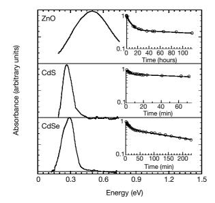
**Figure 4** Infrared absorption spectra of n-type ZnO (4.4 nm), CdS (7 nm) and CdSe (5.4 nm) nanocrystals capped with TOPO. The insets are the corresponding time evolution of the infrared absorbance maximum normalized for comparison. We note that the *x*-axis of the inset for ZnO is in hours.
