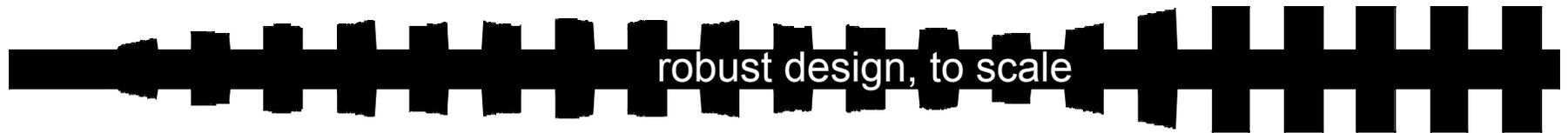
Slow-light waveguide for TE (in-plane polarization), tapers contain **no narrow gaps**, corresponds to contiguous, low-aspect ratio structure in 3d.
