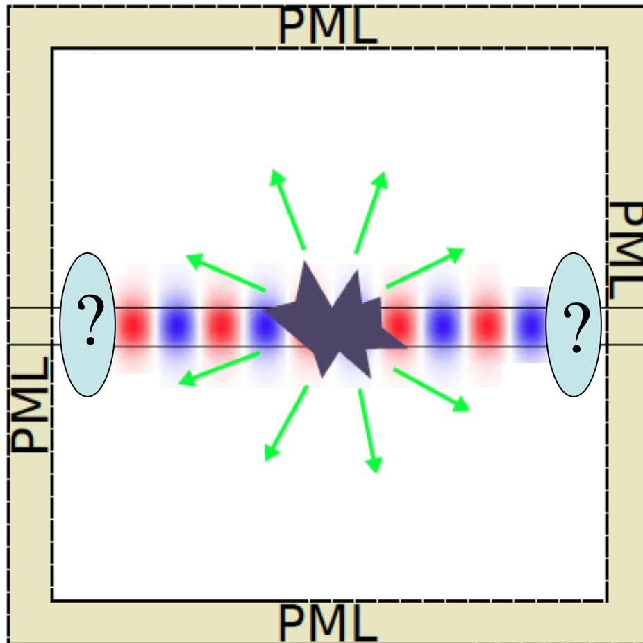
Want some **current source** to excite incident waveguide mode, planewave, etc...
