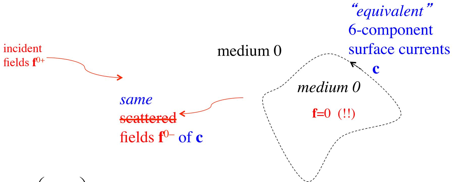
$$\mathbf{f}^0 = \begin{pmatrix} \mathbf{E} \\ \mathbf{H} \end{pmatrix} = \mathbf{f}^{0+} + \mathbf{f}^{0-} = \mathbf{f}^{0+} + \underbrace{\Gamma^0 * \mathbf{c}}_{\substack{\text{convolution with} \\ \text{6x6 Green's function } \Gamma^0 \\ \text{of homogeneous medium 0}}}$$
