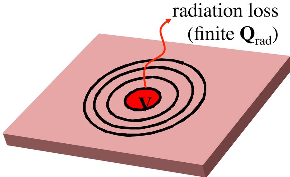
Want some 2d pattern that will **confine light in 3d** with **maximal lifetime** (“ $Q_{\text{rad}}$ ”) and **minimal modal volume** (“ $V$ ”)
