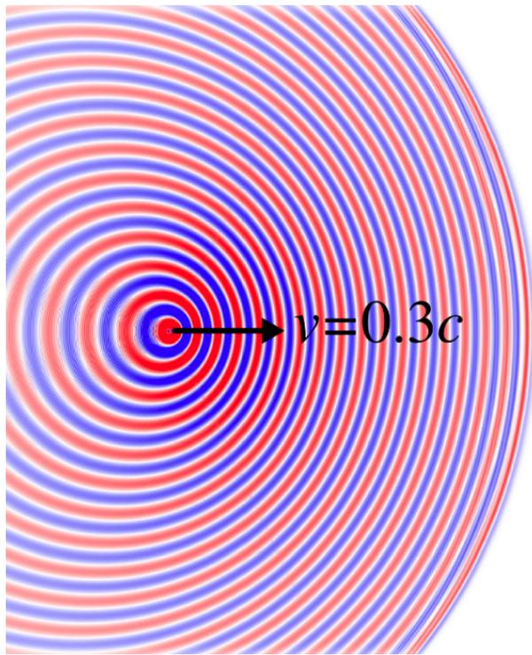
Doppler shift from moving oscillating dipole
