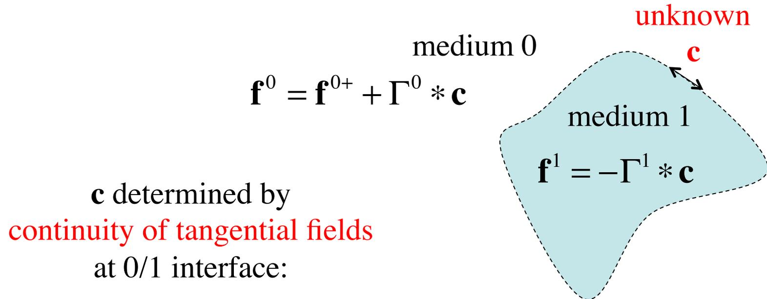
$$\left( \Gamma^0 + \Gamma^1 \right) * \mathbf{c} \Big|_{\text{tangential}} = -\mathbf{f}^{0+} \Big|_{\text{tangential}}$$
