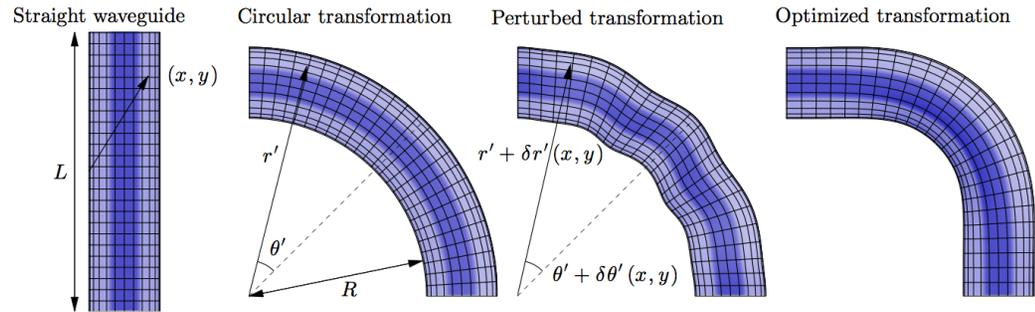
For a given radius  $R$ , **minimize the maximum anisotropy**, subject to index constraints, over “all” transformations  $\mathbf{x}'(\mathbf{x})$ :
