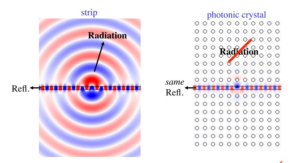
Loss rate ratio = (Refl. only) / (Refl. + Radiation) = 60%  $\checkmark$
