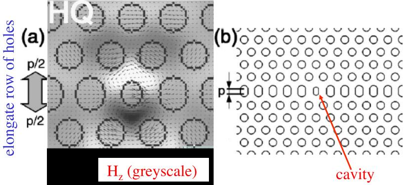
Elongation *p* is a tuning parameter for the cavity... ...in simulations, Q peaks sharply to ~10000 for p = 0.1a(likely to be a multipole-cancellation effect)
