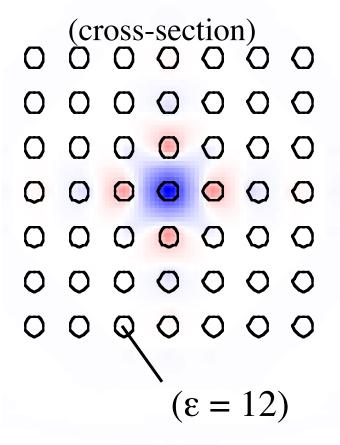
Lower the  $\varepsilon$  of a single rod: push up a monopole (singlet) state.
