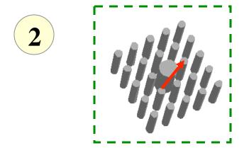
excite cavity with narrow-band dipole source (*e.g.* temporally broad Gaussian pulse)
