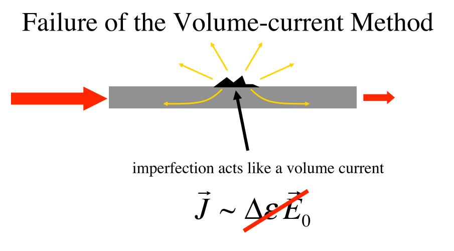
*Incorrect* for large De (except in 2d TM polarization)
