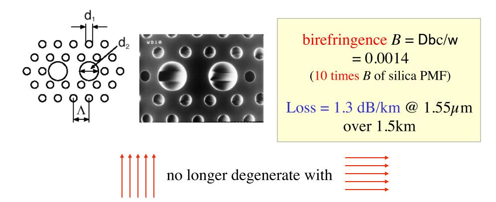
Can operate in a single polarization, PMD = 0 (also, known polarization at output)
