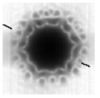
1.7dB/km BlazePhotonics over ~ 800m @1.57µm
