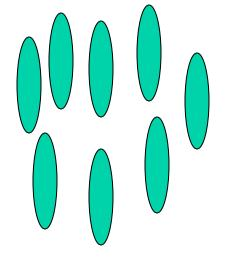
Asymmetric particles oriented by external field: -n on (two) "ordinary" axes can differ from "extraordinary-axis" n by  $\Delta n \sim 15\%$
