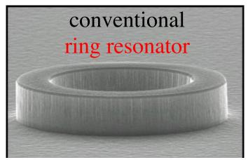
loss limited by disorder (in addition to bending)
