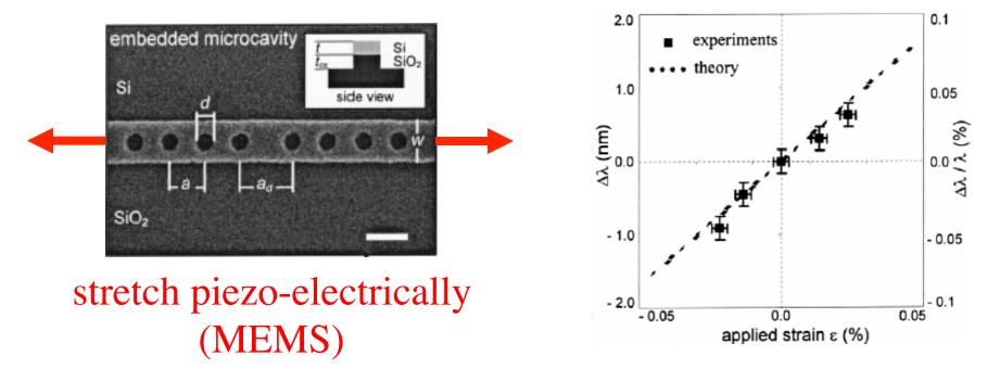
1.5 nm shift @  $1.5\mu m (0.1\%)$ response-time not measured, expected in "microseconds" range
