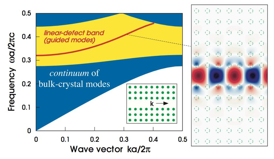
any state in the gap cannot couple to bulk crystal  $\Rightarrow$  localized
