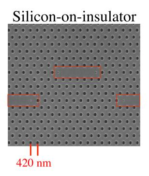
$Q \sim 30,000$ Power threshold ~ 40  $\mu$ W Switching energy ~ 4 pJ
