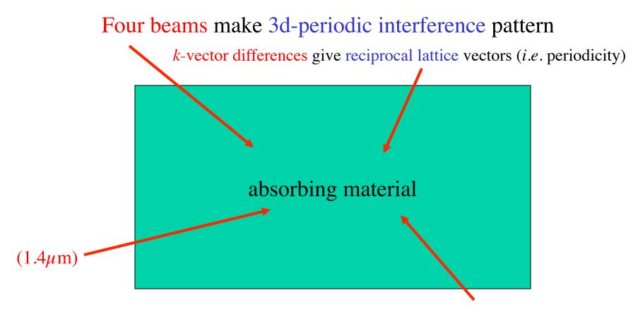
beam polarizations + amplitudes (8 parameters) give unit cell
