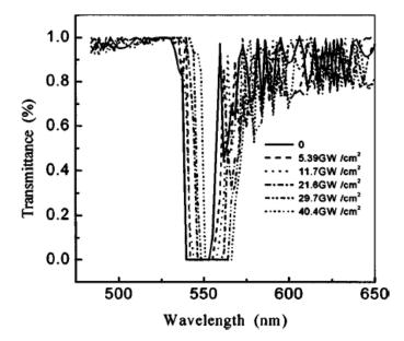
fcc lattice of polystyrene spheres (*incomplete gap*) 13nm shift @ 540nm (2.4%) response time ~ 10 ps
