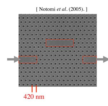
$Q \sim 30,000$ V ~ 10 optimum Power threshold ~ 40  $\mu$ W
