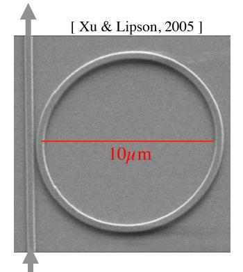
Q ~ 10,000 V ~ 300 optimum Power threshold ~ 10 mW
