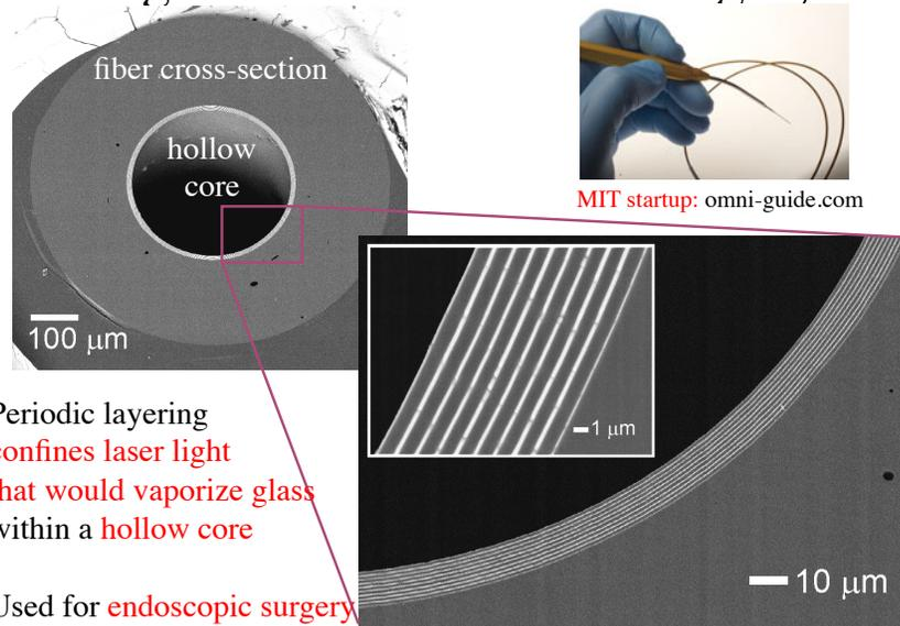
Periodic layering confines laser light that would vaporize glass within a hollow core
