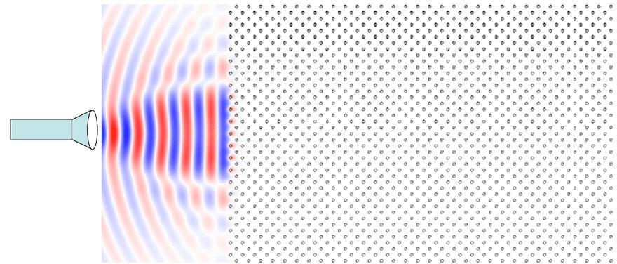
light **cannot penetrate the structure** at this wavelength!
