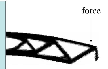
optimized structure, deformed under load
