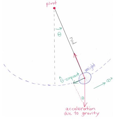
Equation: When the weight is at a certain position, let  $\hat{\theta}$  be the unit vector in the direction that the weight moves as  $\theta$  starts to increase. The  $\hat{\theta}$ -component of the weight's acceleration is
