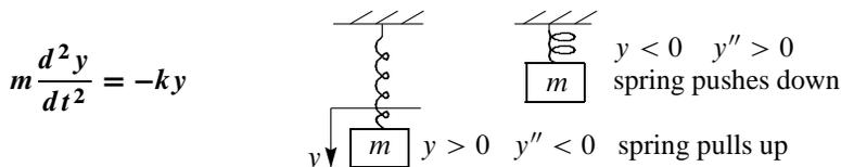
Figure 2.2: Larger  $k$  = stiffer spring = faster  $\omega$ . Larger  $m$  = heavier mass = slower  $\omega$ .
