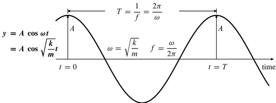
Figure 2.3: Simple harmonic motion  $y = A \cos \omega t$ : amplitude  $A$  and frequency  $\omega$ .
