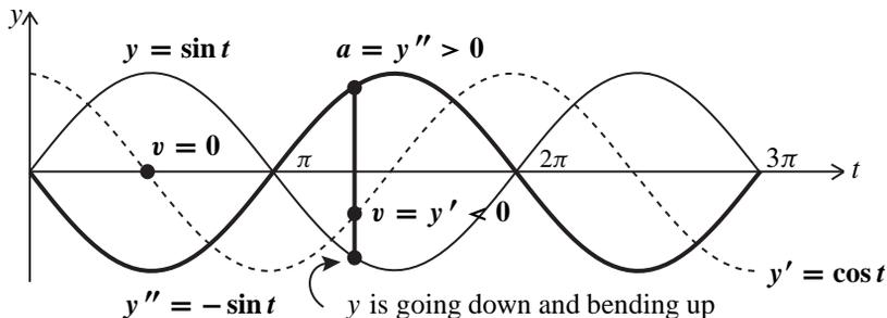
Figure 2.1:  $y'' > 0$  means that velocity  $y'$  (or slope) increases. The curve bends upward.
