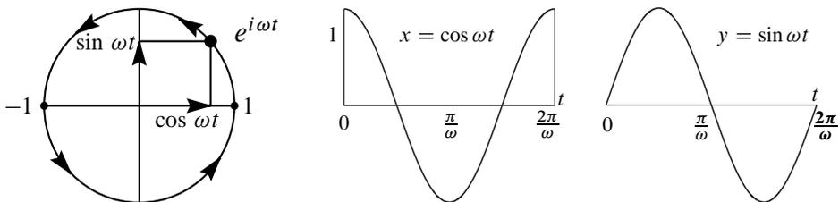
Figure 2.4: Steady motion around a circle produces cosine and sine motion along the axes.
