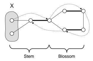
The dotted arcs show a directed path in the auxiliary graph that starts at a vertex in X and ends at a neighbour of set X but does not correspond to an augmenting path. The graph contains flower, which consists of a stem and a blossom. The stem is simply an alternating path and the blossom is an odd-length cycle.
