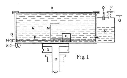
B is the removable plate-glass top which was screwed down with a water-tight joint capable of standing considerable pressure. The tank was 9 inches wide by 12 inches long and 4 inches deep. C is the vertical shaft about which the tank rotates, and D is the driving pulley. The apparatus was rotated at a uniform speed by an electric motor fitted with a governor, but this is not shown in the diagram.
