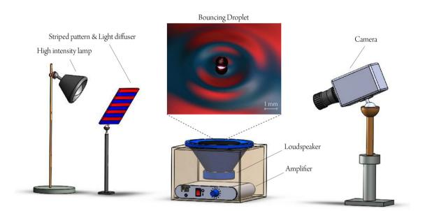
Fig. 1 Schematic of the experimental setup. The striped pattern, reflected from the oil bath, is captured by a camera as a droplet bounces on the interface
