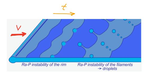
6. At very high speed, shear stresses caused by air induce Happing.
