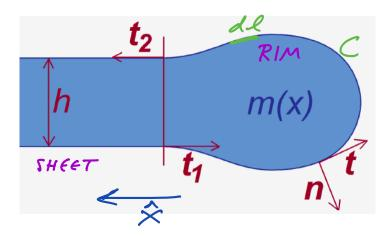
At time t=0, a planar sheet is punchived at x=0 and retracts in the  $\hat{x}$ -direction under the influence of  $F_c=20\,\hat{x}$ .
