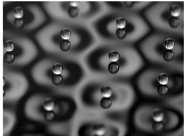
**Fig. 10** A stable lattice of oil droplets formed with our droplet generator bounces on the surface of a vibrated oil bath
