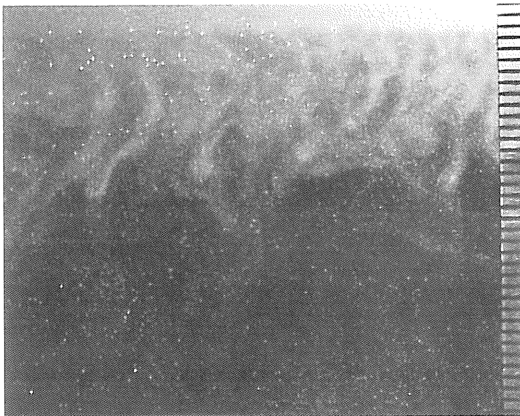
Fig. 5. Photograph of finger convection in a saline-supported layer (Series 2, expt 118); scale increments in mm. Note finger size and the degree of magnification of the image compared with Figs 3a and 6. The photo was taken less than 1 minute after the partition was removed. Finger convection quickly obscured the lower layer and made platform photography futile with the available equipment.
