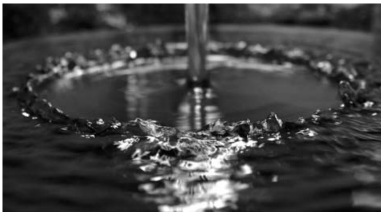
FIGURE 14. The crown-shaped jump arising in a glycerol-water solution of viscosity 5 cS, an intermediary between the polygonal and fully turbulent regimes.
