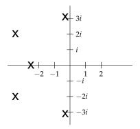
Figure 2: Pole diagram for example 2.
