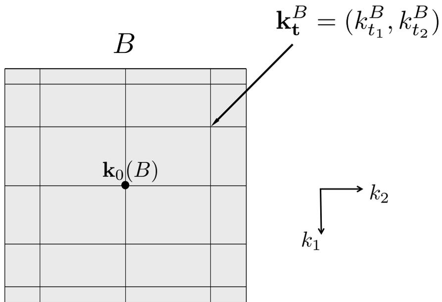
Figure 1: A 2-D,  $q_{k_1} \times q_{k_2}$  ( $q_{k_1} = 7$ ,  $q_{k_2} = 5$ ) Chebyshev grid in box  $B$ .  $\mathbf{k}_0(B)$  is the center of the box.  $\mathbf{k}_t^B = (k_{t_1}^B, k_{t_2}^B)$ ,  $0 \leq t_1 \leq q_{k_1} - 1$ ,  $0 \leq t_2 \leq q_{k_2} - 1$  is a point on the grid.
