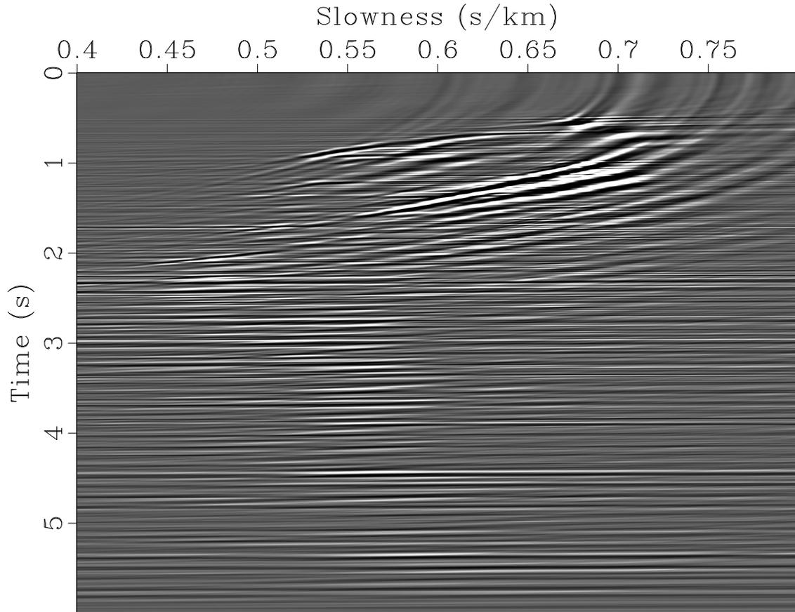
Figure 17:  $N_\tau = 1500$ ,  $N_p = 800$ . Output of the fast butterfly algorithm applied to the field data in Figure 15.  $N = 128$ ,  $q_{k_1} = q_{x_1} = 7$ ,  $q_{k_2} = q_{x_2} = 5$  (here the range of  $\Phi = f\sqrt{\tau^2 + p^2h^2}$  is about 306). CPU time: **6.62 s**.
