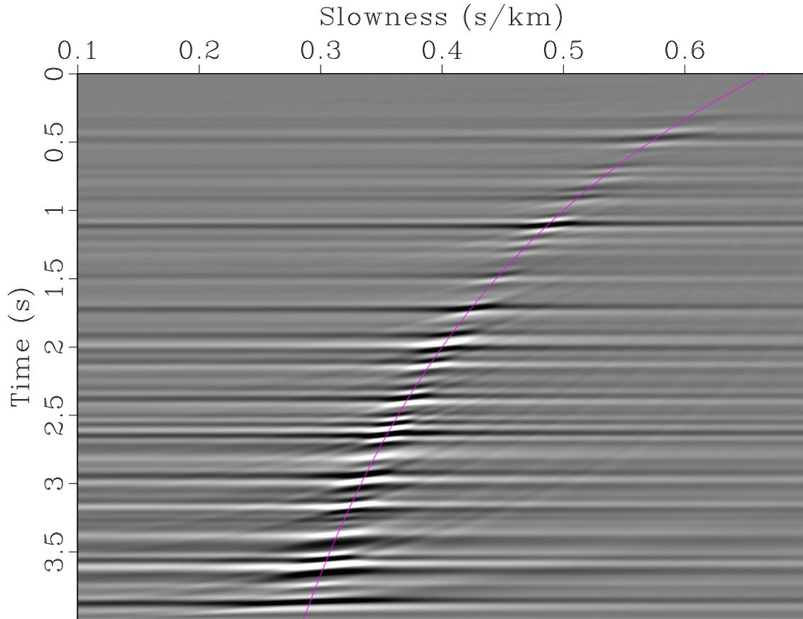
Figure 5:  $N_\tau = N_p = 1000$ . Output of the fast butterfly algorithm applied to the synthetic data in Figure 3.  $N = 32$ ,  $q_{k_1} = q_{k_2} = q_{x_1} = q_{x_2} = 9$  (here the range of  $\Phi = f\sqrt{\tau^2 + p^2h^2}$  is about 125). CPU time: **1.75 s**. Purple curve overlaid is the true slowness.
