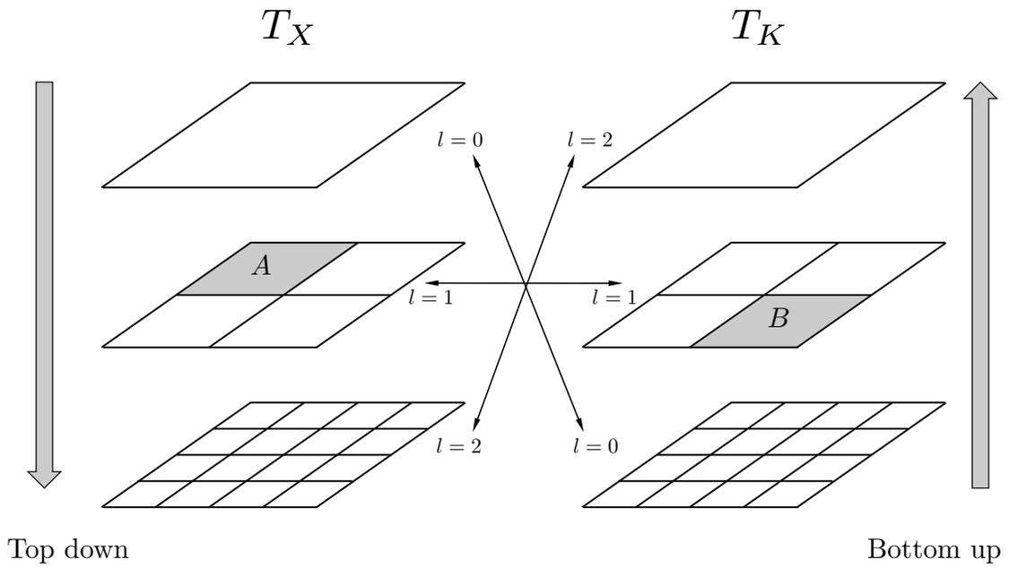
Figure 2: The butterfly quad tree structure for the special case of  $N = 4$ . – **GEO-2013-**
