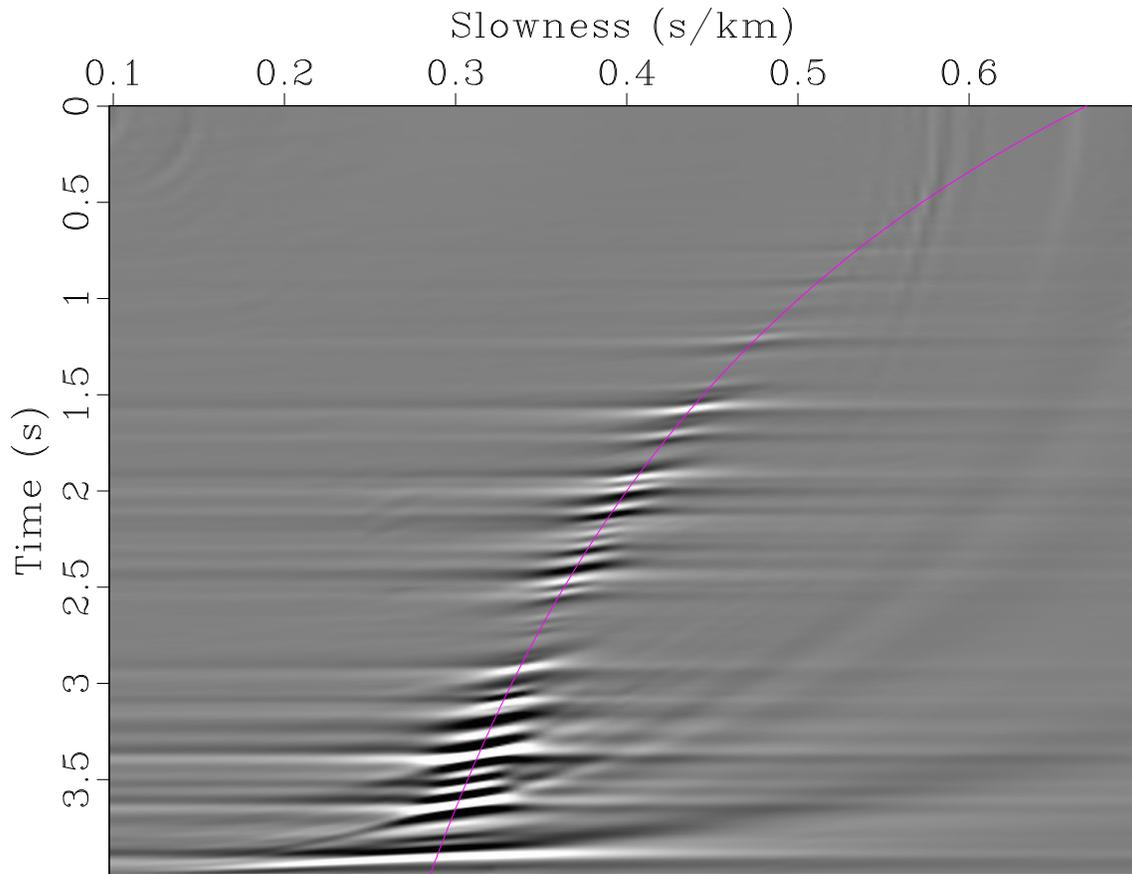
Figure 13:  $N_\tau = 1000$ ,  $N_p = 128$ . Output of the fast butterfly algorithm applied to the synthetic data in Figure 12.  $N = 64$ ,  $q_{k_1} = q_{k_2} = q_{x_1} = q_{x_2} = 5$  (here the range of  $\Phi = f\sqrt{\tau^2 + p^2(h_1^2 + h_2^2)}$  is about 162). CPU time: **1.67 s**. Purple curve overlaid is the true slowness.
