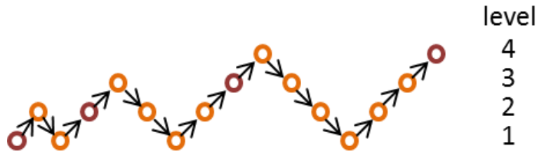
Figure 4: Full Multigrid Algorithm 1 V-cycle per refinement
