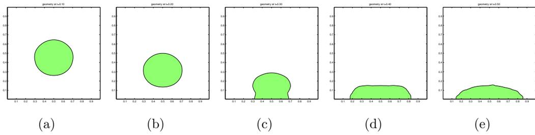
**Figure 3:** Evolution of a water drop with surface tension. Drop remains circular as it hits the base;  $Re=10$ ,  $B=1/800$ , density ratio  $1/1000$ , grid  $90 \times 90$ .
