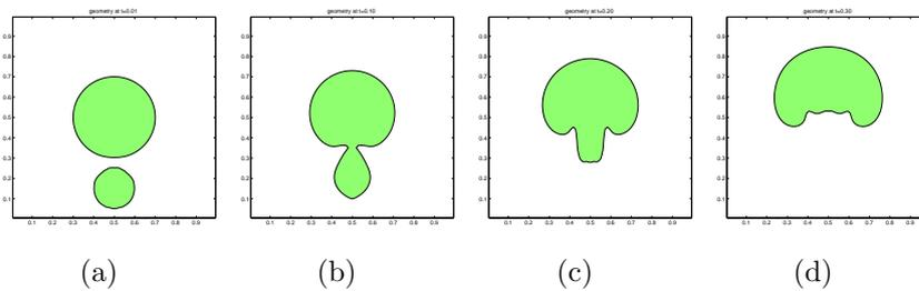
*Figure 2: Bubble merge;  $Re=100$ ,  $B=200$ , density ratio 1000/1, grid  $90 \times 90$ .*
