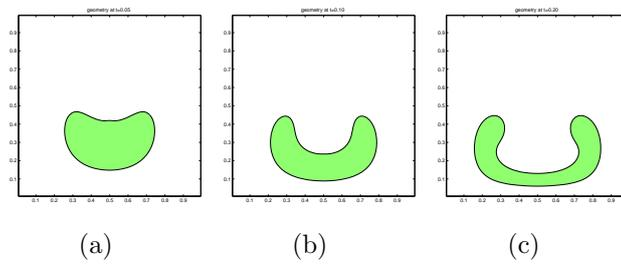
**Figure 5:** Evolution of a droplet without surface tension.  $Re=10$ ,  $B=Inf$ , density ratio  $1/2$ , grid  $90 \times 90$ .
