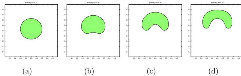
*Figure 1: Bubble rising with medium range Reynolds number;  $Re=100$ ,  $B=200$ , density ratio 1000/1, grid  $90 \times 90$ .*
