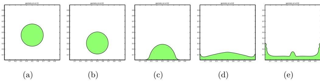
**Figure 4:** Evolution of a water drop without surface tension.  $Re=10$ ,  $B=Inf$ , density ratio  $1/1000$ , grid  $90 \times 90$ .
