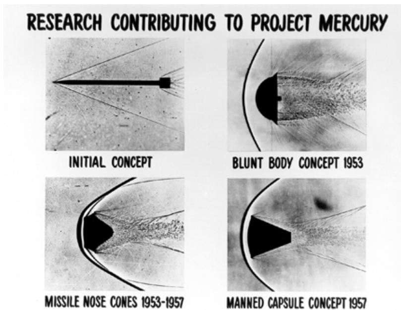
An innovative idea by Dr. Julian Allen in 1953 proposed that a blunt body would be able to withstand a more intense reentry profile. The reason for this is that the shock wave becomes detached from the nose of the vehicle and forms a *bow shock* as shown in the three other plots above. A bow shock wave serves to decrease the severity of the atmospheric friction by diverting some of the flow away from the vehicle. All spacecraft use blunt-body geometry to survive reentry.
