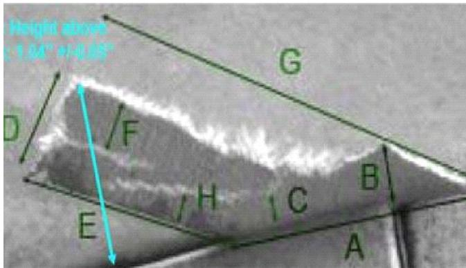
To determine the possible damage a protruding piece of gap filler could cause, a simulation was performed in which a 2 inch thick object protruded 4 inches from the underside of the shuttle. The gap filler is located on a portion of the vehicle that is designed to experience moderate heat.
