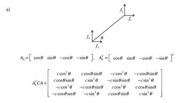
b) To  $A_0^T y = f$  be solved, external forces f's should uniquely determine internal bar forces w's and vice versa (without inducing instabilities in u). Therefore, the external forces should be matching tensile forces or compressive forces acting opposing ends of the bar. The external forces f's should have form of
