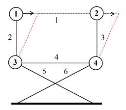
For this case, there are only horizontal motion at hinge 1 and 2, and no motion for other hinges.
