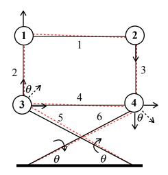
For this case, hinge 3 and 4 rotate along bar 5 and 6 while hinge 1 and 2 vertically translate as the same amount as hinge 3 and 4 respectively.
