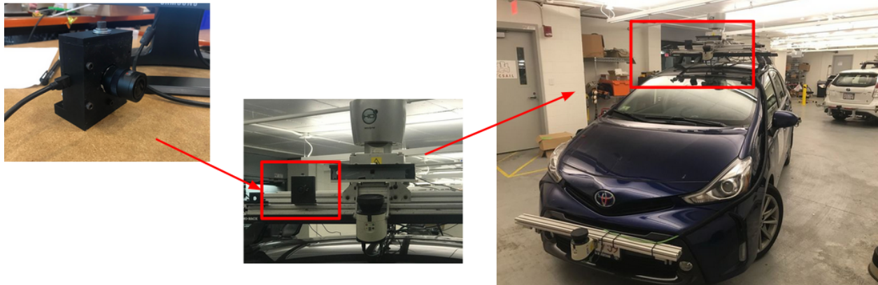
Figure 2: DAVIS240 sensor position on the vehicle
